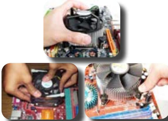
*Gambar Pemasangan Heatsink/Fan processor.*
